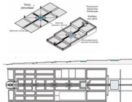
**Figure 1.** "Chor-bog" traditional water structures. Irrigation of "garden": a) horizontal surface in the plain; b) perimeter construction; c) relief plane, at a slope of 2-10%.
