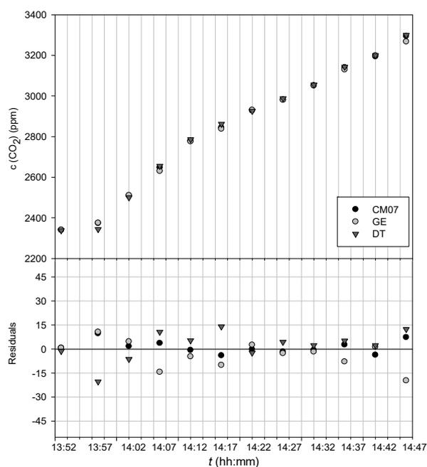
**Figure 2.** The CO<sub>2</sub> concentrations measured by our three instruments (accuracy for CO<sub>2</sub>; CM07 ± 30 ppm ± 5 % of reading (0-5000 ppm); GE ± 50 ppm; DT ± 8 % (2000 - 9999)) in a wide range of CO<sub>2</sub> concentrations. The lower graph shows residuals from the mean values (in ppm)
