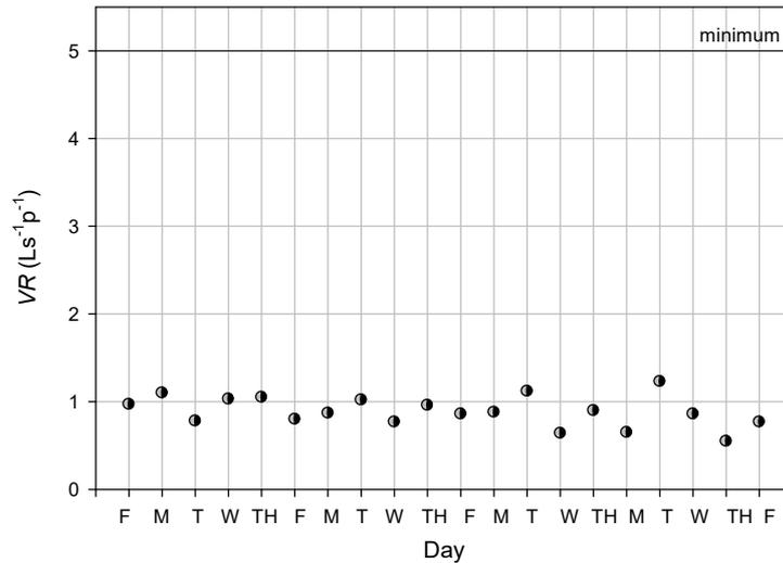
**Figure 7.** The calculated ventilation rates for all days were considerably below the ASHARE and EN13779 minimum recommended value
